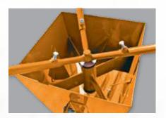
Hopper is equipped with angled baffles to gently and evenly direct grain onto the chute.
